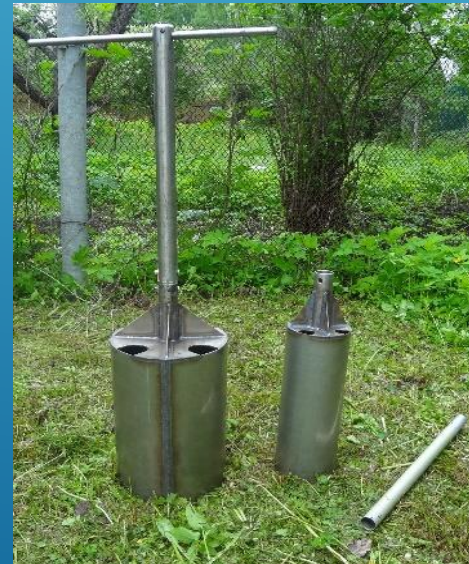
screw for the installation of lysimeters
